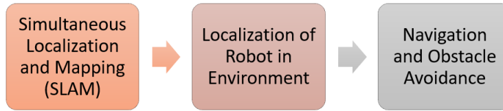
Figure 1: Typical workflow of preparing a robot for autonomous navigation
